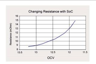
Typical internal resistance readings of a lead acid battery
