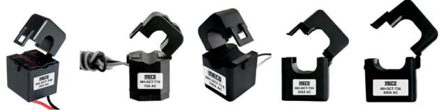
MECO Split Core Current Sensor's are designed for fast and easy installation. Split Core Current Sensor's are ideal for installation on existing electrical wiring by snapping around the conductor. This method permits safe, easy and portable current measurement. These sensors are small in size and have a secure locking hinge. The Sensor's have a high secondary to primary turn ratio.
