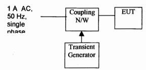
Transients generated by the generator were coupled to the 230 VAC Supply through a coupling N/W.
