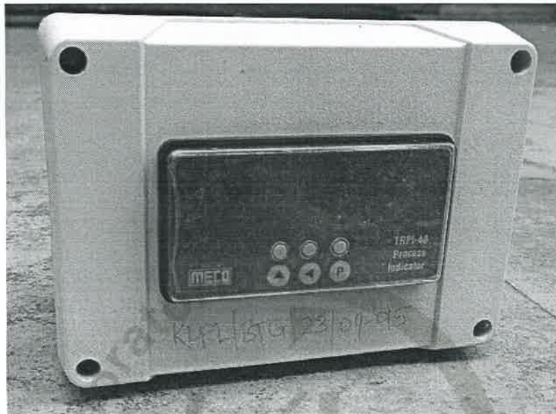
Picture1: 4 Digit Triple Range Programmable Process Indicator
