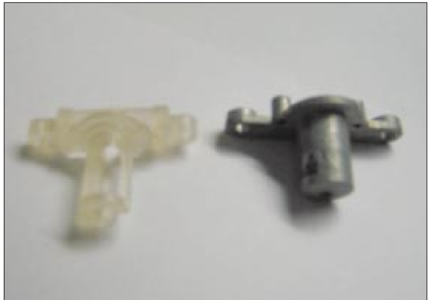
Plastic vs zinc diecasting of an internal moving iron meter part
