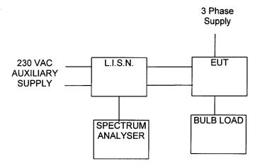
Measurements carried out on Auxiliary Mains while the measurement circuit energised by 415 V 3  $\phi$  supply and carrying 5 A current
