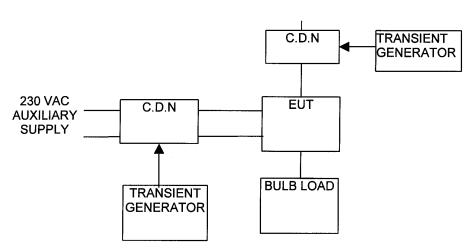
Conducted Immunity tests were carried out by coupling transients generated by generator, separately on 230 VAC Auxiliary supply and 3 Phase I/P through a CDN. The test set-up is as shown in the figure above. EUT performance was evaluated as per the following:-
