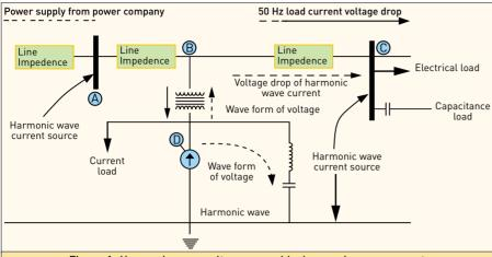
Figure 1: Harmonic wave voltage caused by harmonic wave current
